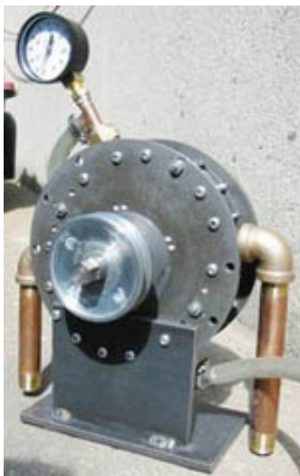
Steam Engine: A steam powered Quasiturbine.
