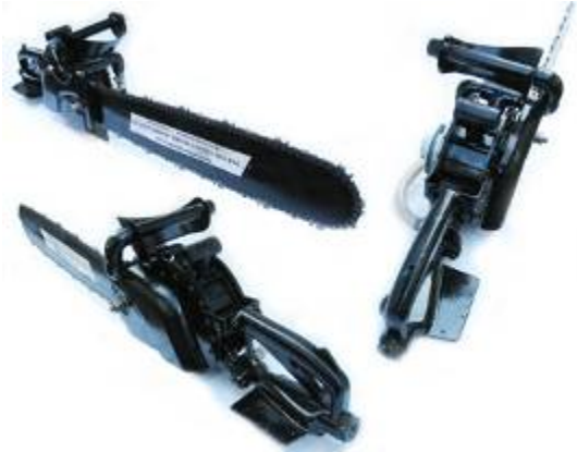
Hand-Tools: A pneumatic chainsaw concept prototype using a Quasiturbine motor.
