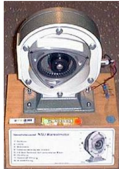
Wankel: Uses counter seal w/ variable rotation angle.
