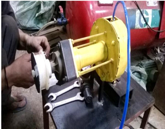
Photo 1:- Photo of Quasi turbine rotary air engine
