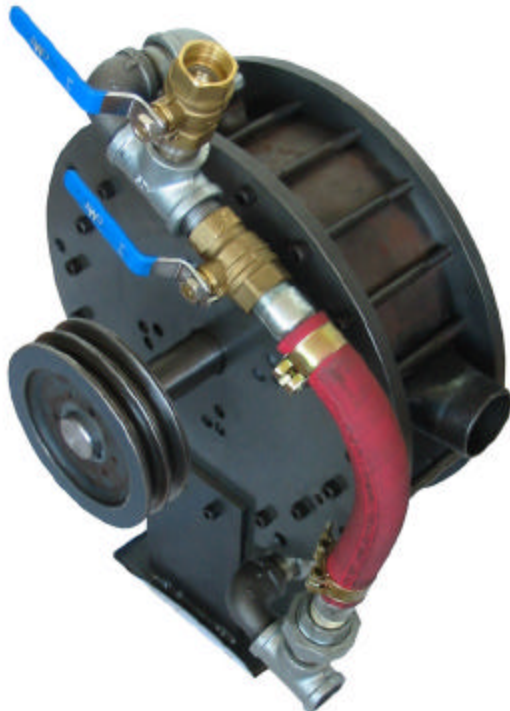
Figure 5. Photo of a Steam Quasiturbine Model QT5LSC, having 600 cc per chamber, and expanding 4.8 liters per revolution. The rotor diameter is 21 cm (11 inches), by 11 cm (4 inches) thickness. Idle with only 1/15 of a bar (1 psi).
