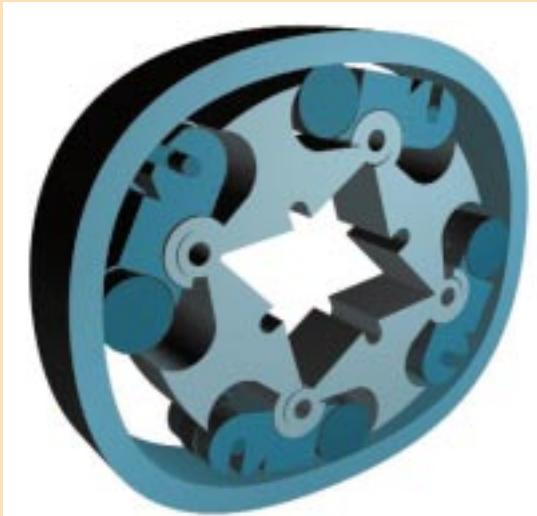
An engine at different phases of rotation showing how the rotor and carriages match the complex internal profile of the combustion chamber. An animation can be seen on the Internet at [www.quasiturbine.com](http://www.quasiturbine.com)
